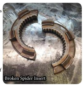
Step 8: Check the spider insert for cracks or total breakage. If broken replace with our high strength version #50-338. If rubber damper is damaged, replace with #50-337.
