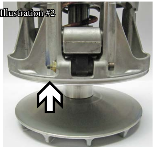
Install weight pin with the nut on the LEFT side of the clutch.
