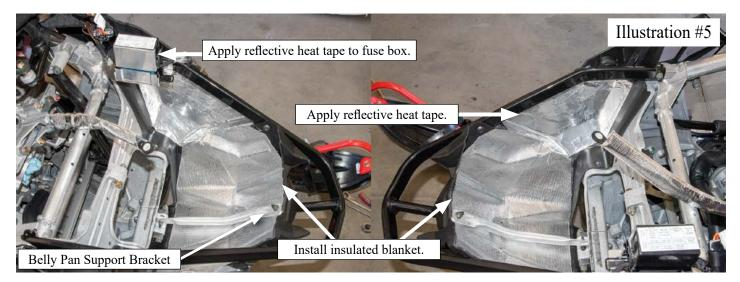
**Step 9:** Apply heat tape near the exhaust outlet of the belly pan shown in Illustration #7.
