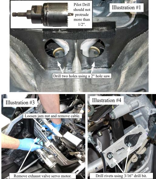
move the fuse box from fuse box bracket by lifting up on the black safety tab and sliding the fuse box towards the center of the sled. Remove the fuse box mounting bracket from the bulk head cross member by drilling out the rivets using a 3/16" drill bit. (Illustration #4). The stock fuse box mounting bracket will not be reinstalled.
