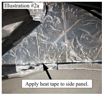
**Step 8:** Disconnect speedo wire plug. Slide insulated heat sleeve onto speedo wires. Reconnect plug and straighten the insulated sleeve so that it covers the speedo wires completely in the exposed areas from the bottom side of the chaincase to the top front of the chaincase. Use zip ties to tie wires to the chaincase. Apply heat tape to the recoil housing, chaincase fill cap and tube (see Illustration #5).
