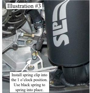
**Step 5:** Install spring clip onto bulkhead in the open threaded hole on the right side of the bulkhead with supplied 8 x 1.25 x 20mm bolt with a dab of blue thread lock. Rotate it to the 1 o'clock position (see illustration #3).
