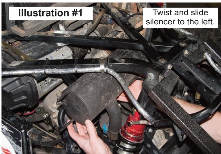
3. Remove the stock exhaust inlet U-tube from the machine by disconnecting the retaining springs and removing the U-tube from the left side of the machine.
